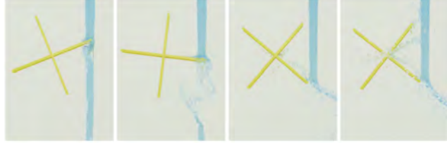
Fig. 15. Water wheel. In this two-way coupling example, water flows down onto a wheel, making it spin. Our approach evaluates the forces involved in this interaction five times faster than the work of Bogner [2017].
