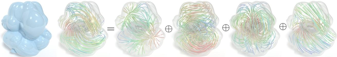
Fig. 5. **Hodge-Morrey-Friedrichs decomposition.** For any 3D bounded domain, a vector field can always be decomposed into the orthogonal sum of the gradient of a scalar field vanishing on the boundary, the curl of a normal field, a tangential harmonic fields, and a harmonic gradient field.
