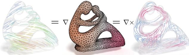
Fig. 11. **Potentials for the exact and coexact field.** In any 3D volume, the fifth vector component  $\eta$  in our decomposition (left) can be expressed both as a gradient field (middle) and a curl field (right).
