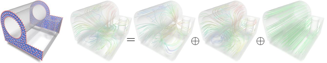
Fig. 12. **Mixed boundary conditions.** Our orthogonal decomposition extends naturally to mixed boundary conditions as well; in this example, no constraints are set on the blue regions, but tangential conditions are set on the rest of the boundary.
