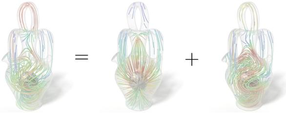
Fig. 2. **Helmholtz decomposition.** Vector field in a vase with a spherical cavity decomposed into a gradient and a curl field, but with a nonzero  $L_2$  inner product between these two resulting components.
