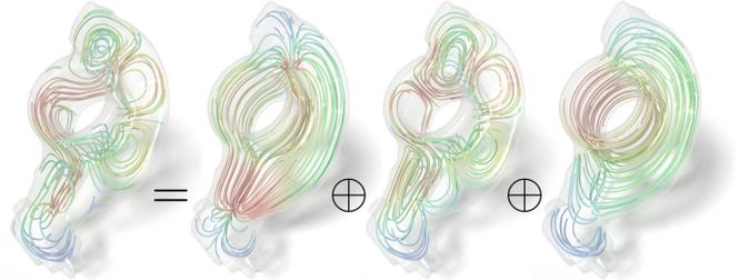
Fig. 4. **Helmholtz-Hodge decomposition.** On this example, a tangential field is decomposed into the orthogonal sum of a tangential gradient field, a tangential curl field, and a tangential harmonic field.
