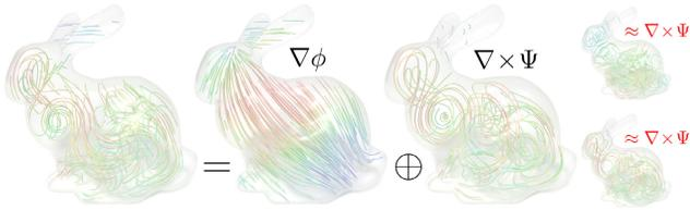
Fig. 13. **Non-diagonal Hodge star.** Even for higher-order accurate Hodge stars, our decomposition still only requires sparse linear systems. Using a diagonal  $S_1$  in the Laplacian produces inaccurate potentials (right), whether we use a curl operator with a diagonal (top) or non-diagonal (bottom)  $S_1$ .
