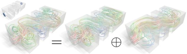
Fig. 14. **Decomposition of a channel flow simulation.** For a simulated channel flow (inlet and outlet in blue), the resulting vector field is decomposed into a curl field and a harmonic field, with the blue regions are set as unconstrained and all other boundary regions as tangential.
