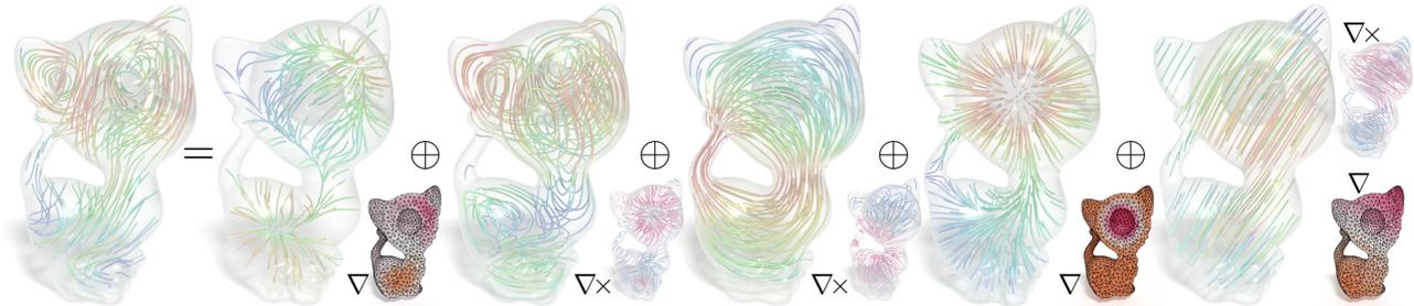
Fig. 1. **Five-Component Vector Field Decomposition.** On a tetrahedral mesh of the kitten with a spherical cavity, a vector field is decomposed into a gradient field with zero potential on the boundary, a curl field with its vector potential orthogonal to the boundary, a pair of tangential and normal harmonic fields, and a harmonic field that is both a gradient and a curl field. Potential fields are shown in the corners of their corresponding components.
