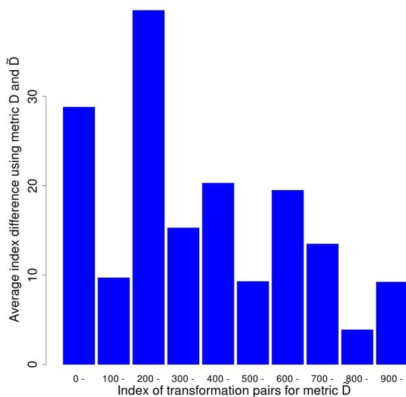
Figure 5: The distribution of error when ignoring the non-uniqueness. Each interval contains 100 successive transformation pairs. The index difference is random and small relative to the range (1000).
