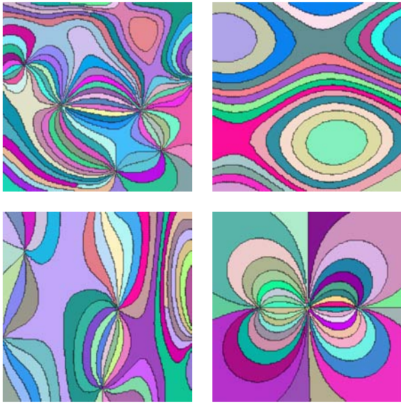
Figure 1: Variational Segmentation: Error-driven clustering is performed on various flow fields using the L^2 metric for vector comparisons. Each color represents an area in which both direction and magnitude of the field is very similar, providing an otherwise hidden insight into the system.
