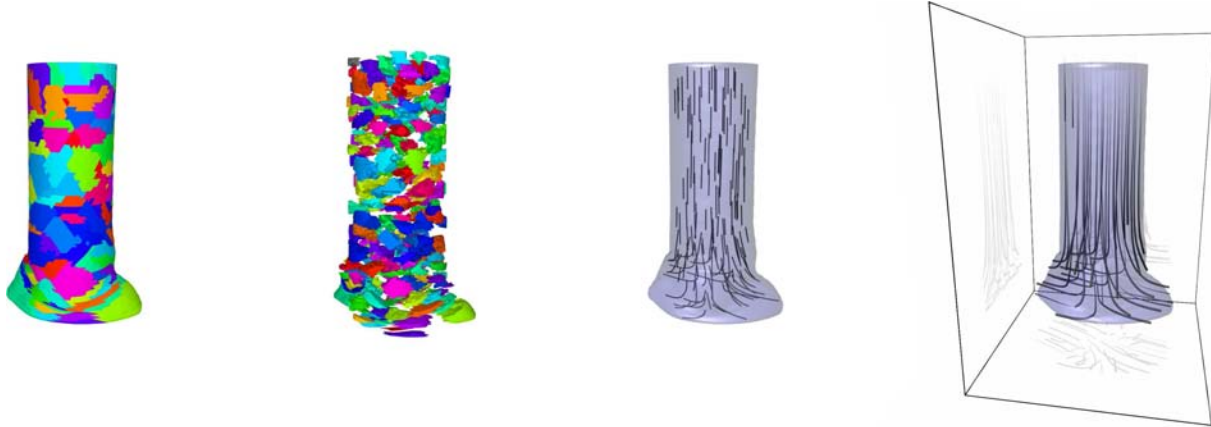
Figure 5: Pipeline for visualizing a cylinder dataset during impact under non-slip conditions, 100k tetrahedra. Left: Variational segmentation into 200 regions. Middle-Left: Exploded view of the cluster volumes. Middle-Right: Streamlines initiated from the centroid of each cluster, terminated at the region boundary. Right: Thinning tubes drawn through the entire domain while adhering to a distance threshold. We use orthogonal shadows projected on the base planes for added 3D cues.
