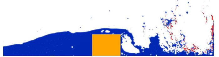
**Fig. 5: Velocity-limiting adaptive viscosity I.** In this turbulent two-phase example (liquid in blue), regions where our velocity-limiting adaptive viscosity is turned on to prevent potential blowups are highlighted in red, demonstrating its spatial sparsity and proving that its impact on the overall flow structure is typically negligible.
