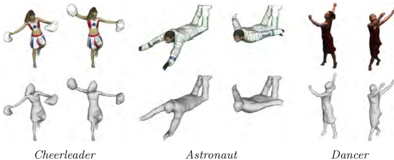
Fig. 6. Results of our approach for the Cheerleader , Astronaut and Dancer sequences. Comparison between the original visual hull reconstruction (top) and the temporally consistent mesh (bottom).
